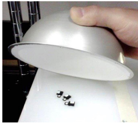
Figure 2. Zeroing the OSLDs with an x-ray light box. The integrating sphere, when placed on top of the OSLDs, multiplies the light fluence incident on the dose-sensitive material.
