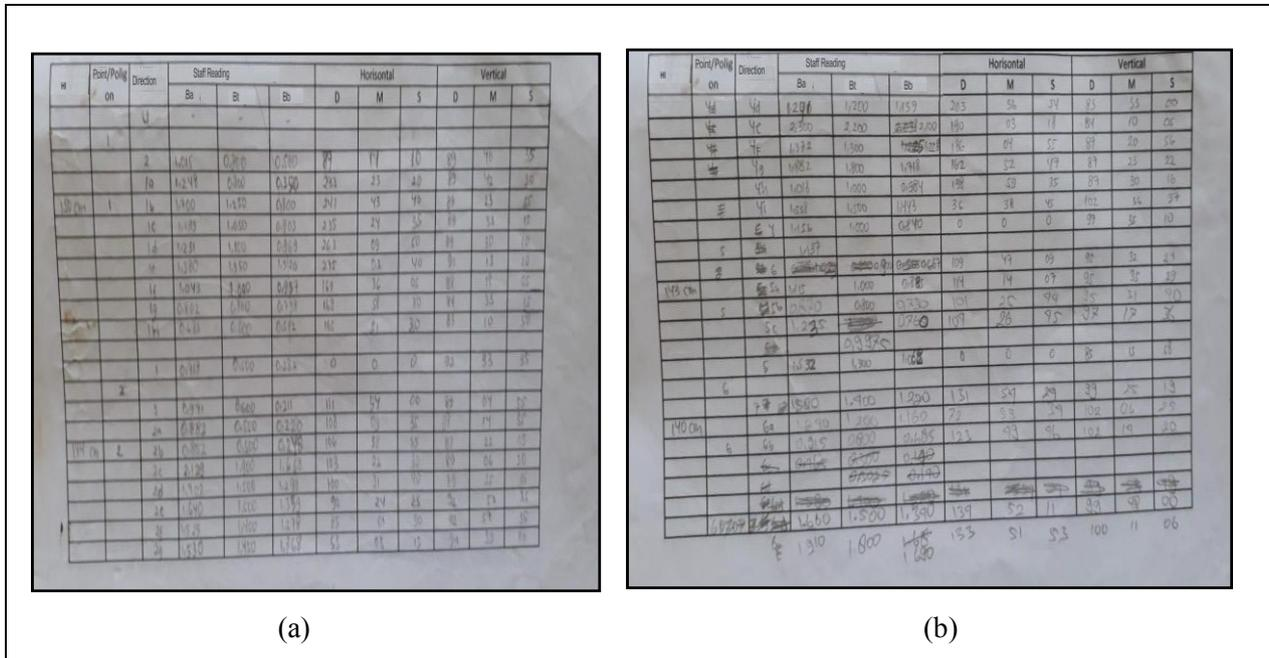
**Figure 1.** Conventional field notes of topographic measurement: (a) first sheet and (b) third sheet, both of them showing inconsistencies in legibility, in third sheet is less legible than first sheet.
