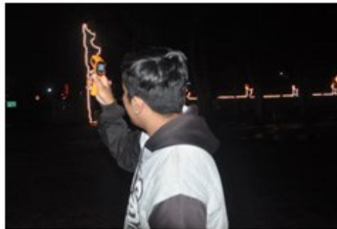
Figure 6. Surveyor measures of spot temperature of overhead light source.
