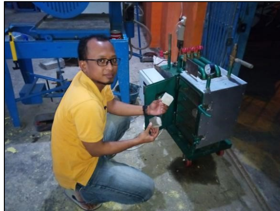
Figure 6. Curing of mortar with steam.
