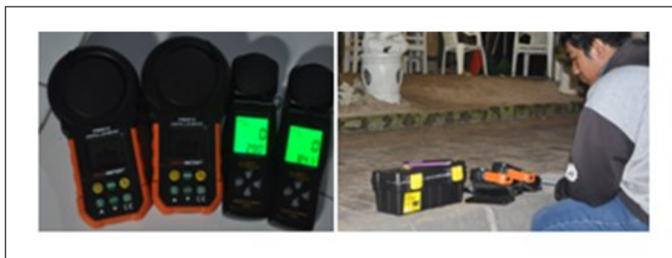
Figure 5. Lux meter uses MS6612 and AS802 model and action of sampling.
