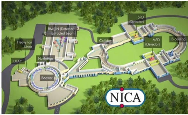
Figure 1. Layout of accelerating facility NICA [1].
