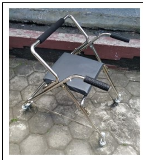
Figure 2. Design and prototype walker trainer.
