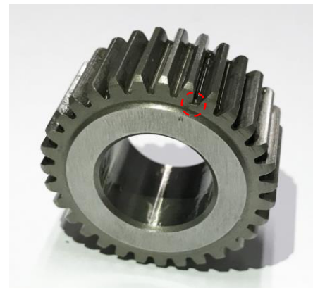
Figure 9. The cracked tooth on planet gear.
