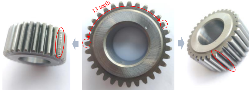
Figure 13. The worn surfaces with interval of 13 teeth on the planet gear.
