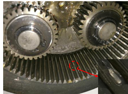
Figure 15. The spalled tooth on the ring gear.
