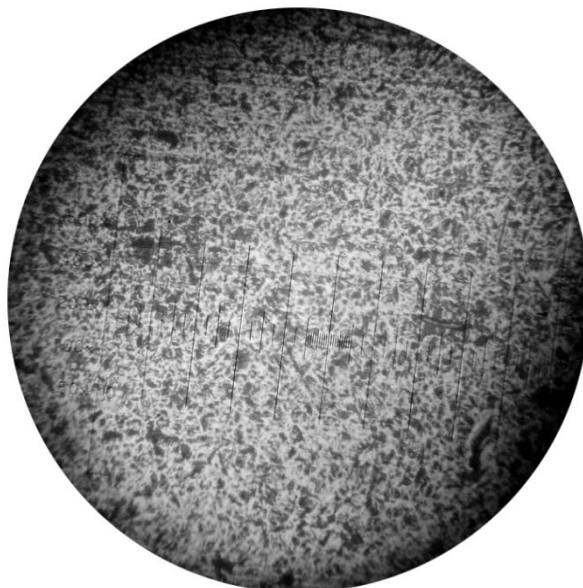
Figure 3a. Structure of steel 65G after the first cycle (increase in X500)
