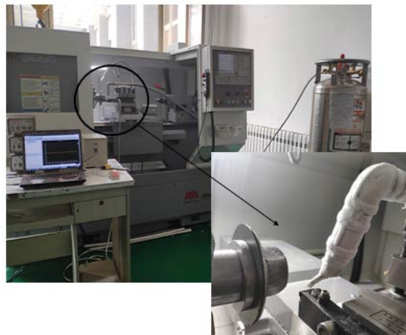
Figure 1. Testing apparatus of cryogenic cutting
