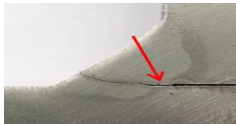
Figure 4. A Typical Crack Location of T-joint
