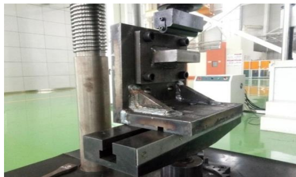
Figure 2. Fatigue Testing Machine
