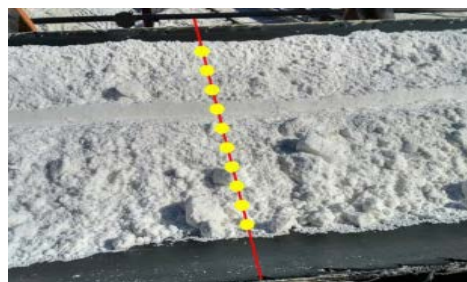
Figure 1. Laser Triangulation Method for Measuring Surface Height
