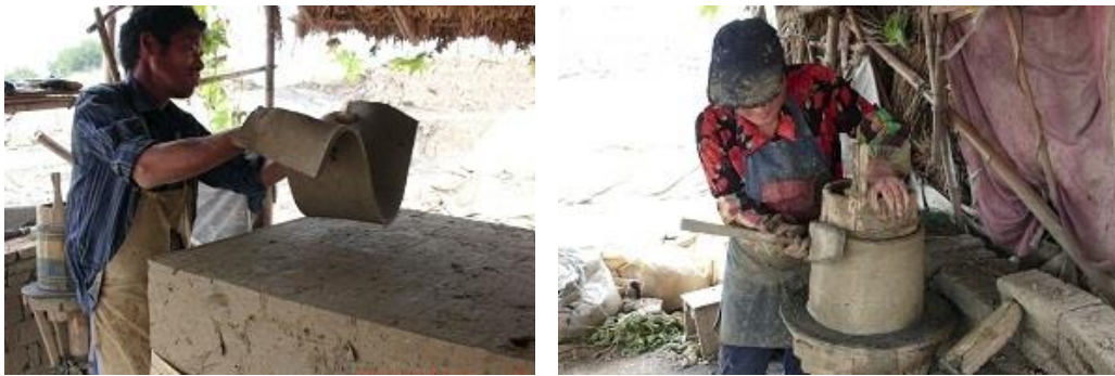
Figure 3. Traditional Production Process of Unburned Tile
