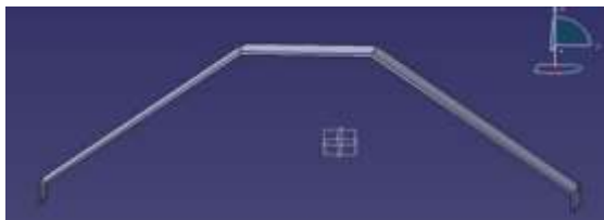
Fig.1. 3D Model of the landing gear using CATIA
