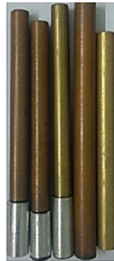
Fig 3: Experimentation on EN8 with Al6061+SiC(3%,6%,9%), Copper and Brass tools
