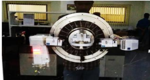
Figure.4.2 XRD Setup
