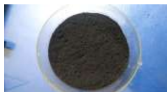
Fig 2. Acidified neem saw dust
