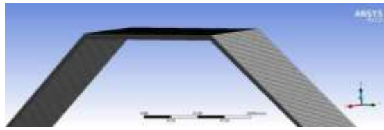
Fig.2. Hexahedral meshing of the landing gear part
