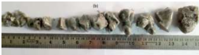
Fig.3 The particles size for both Air quenched (a) \text{CaO-Fe}_2\text{O}_3 and (b) \text{CaO-B}_2\text{O}_3
