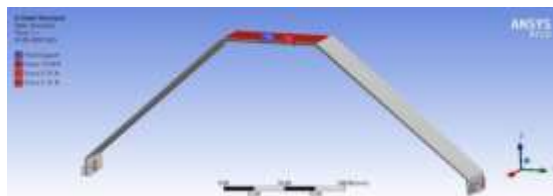
Fig.3. Loads action on the landing gear along positive and negative z-axis
