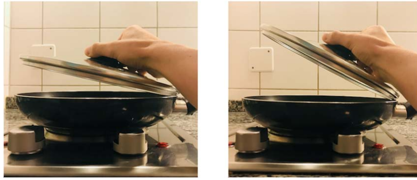
Figure 1. The ‘Helmholtz pan’ with lid at 10° (‘closed’, left) and at 30° (‘open’, right).
