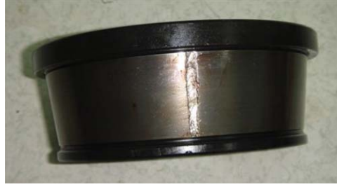
Figure 15. The bearing with a defect on the inner race.
