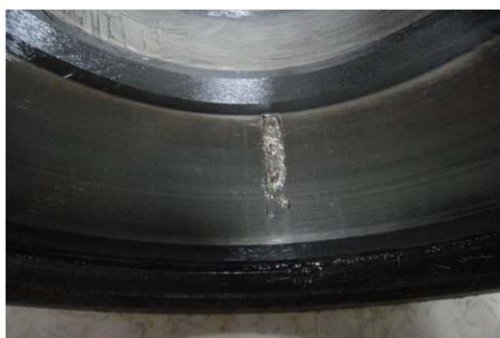
Figure 20. The bearing with a defect on the outer race.
