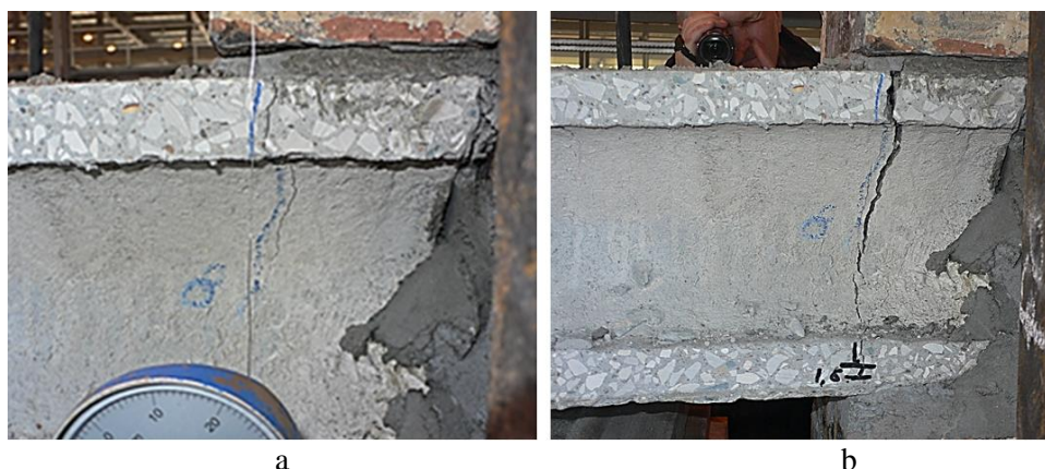
Figure 4. Cracks in the restraint zone of sample №1. a - at load F = 22.8 kN (crack opening width up to 0.2 mm); b - at load F = 41 kN (crack opening up to 7.0 mm).
