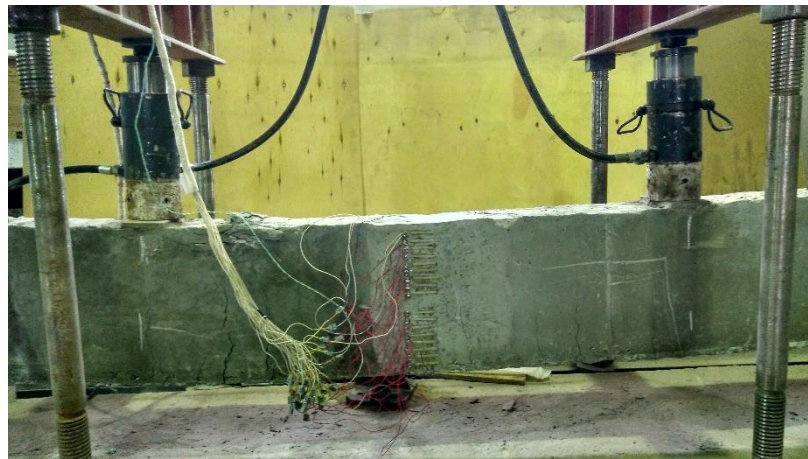
Figure 5. View of the sample under load after failure
