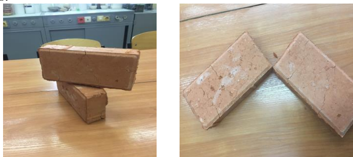
Figure 4. Samples of ceramic pavers based on the raw clay composition are talc rock.
