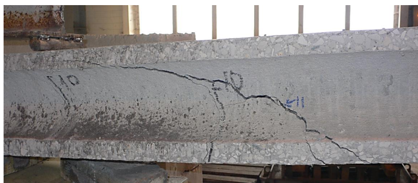
Figure 11. Normal and inclined cracks in sample № 6 at load F=41 kN.
