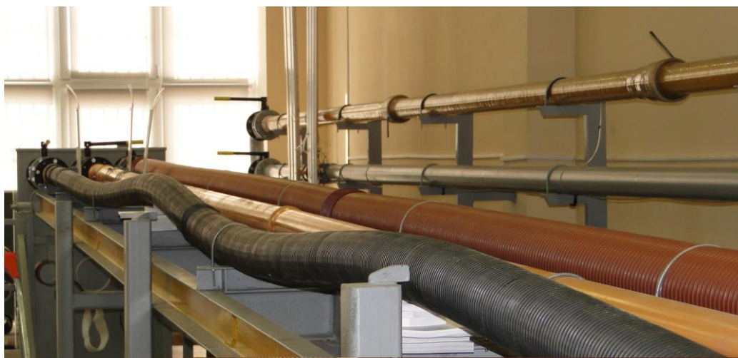
Figure 3. Hydraulic stand with a deflected pipeline of two-wave configuration
