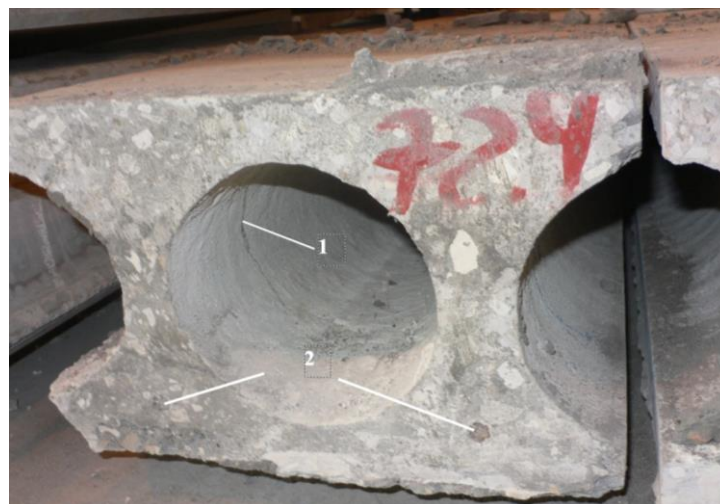
Figure 12. State of the supporting parts of the samples dismantled after testing. 1 - normal crack near ground; 2 - cores.
