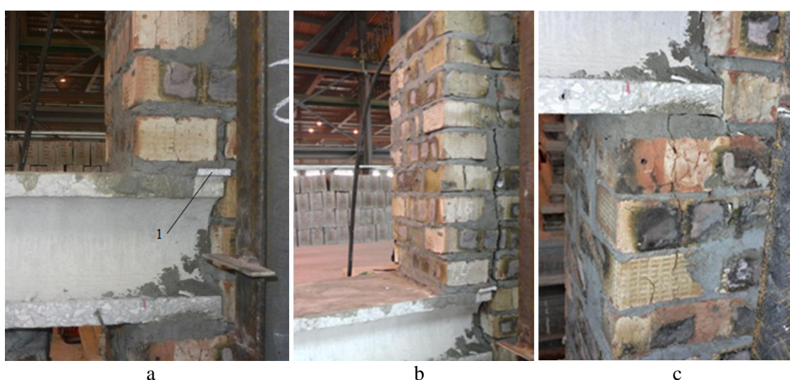
Figure 8. Support area of sample № 4. a – before loading; b - at a load of 41 kN (over the sample); c- at a load of 41 kN (under the sample); 1 - soft gasket.
