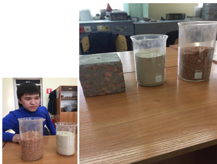
Figure 1. General view of a chemically active filler, thermolitic sand and concrete sample based on them for a pile foundation.
