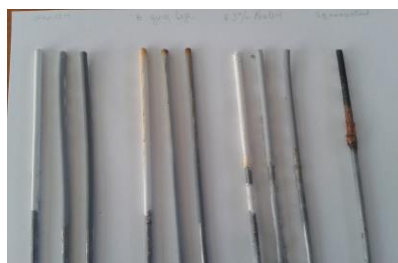
Figure 11. Test results of steel rods in various environments..
