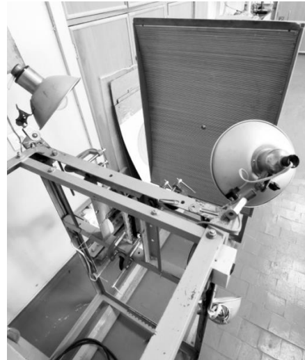
Figure 4. Fixing the beam model in the power frame of the installation.
