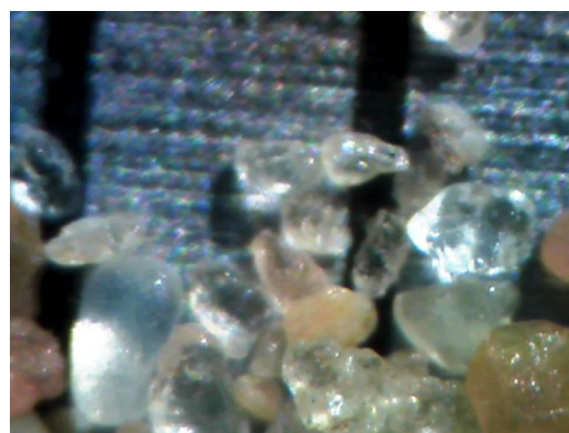
Figure 2. Ordinary Volga river sand under a microscope (scale 1 mm.)
