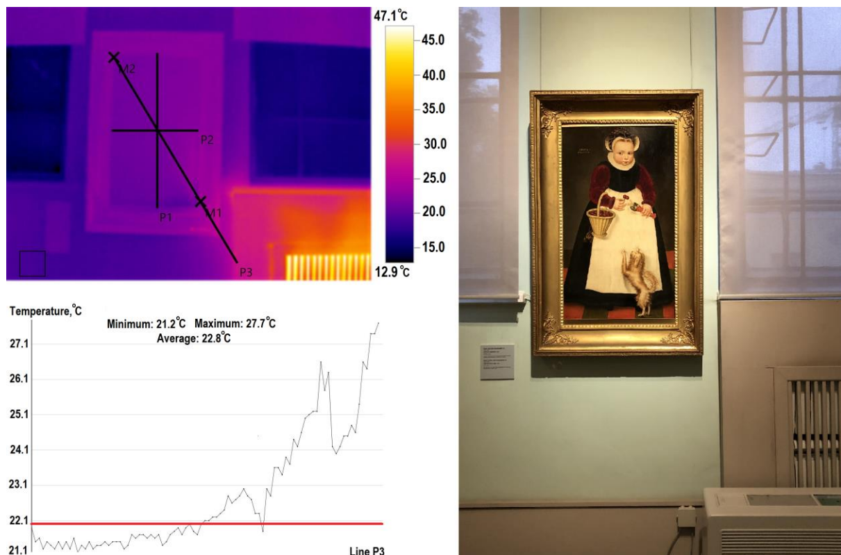
Figure 2. The results of experimental studies (exhibition hall 1). Left top picture – thermographic image; bottom left picture – temperature curve (line P3); right picture – photo of exhibit.
