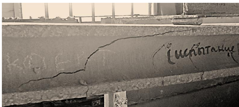
Figure 9. Normal and inclined cracks in sample №. 5 at load F=41 kN.
