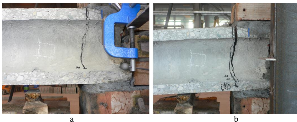
Figure 7. Cracks in the restraint zone of sample №3. a - at load F=19.4 kN (crack opening width up to 0.5 mm); b - at load F=38.8 kN (crack opening up to 10.5 mm)
