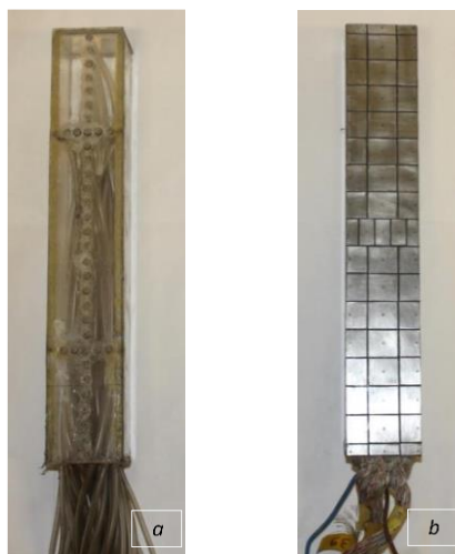
Figure 2. General view of the building model for measurements: a – pressure, b – heat transfer coefficient.
