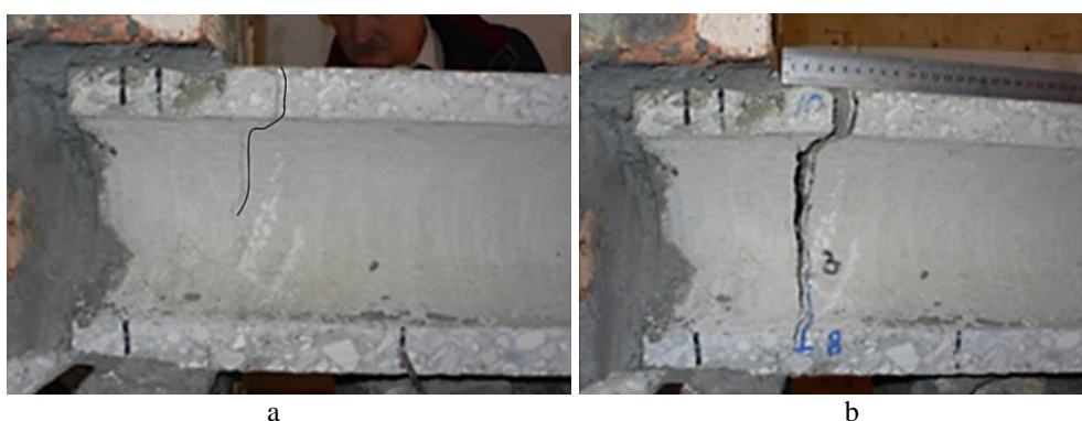
Figure 10. Cracks in the restraint zone of sample № 6. a - at load F=15 kN (crack opening width up to 0.2 mm); b - at load F=41 kN (crack opening width up to 12 mm).
