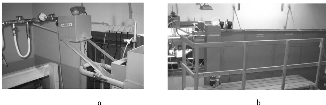
Figure 1. Experimental stand: a – rapid mixing chamber; b – mechanical and contact flocculation tanks and settlement tanks.
