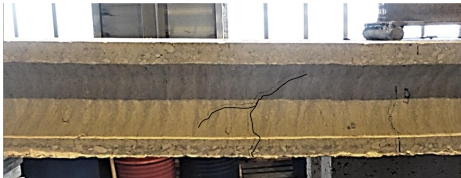
Figure 6. Normal and inclined cracks in sample №2 at load F=26.9 kN.
