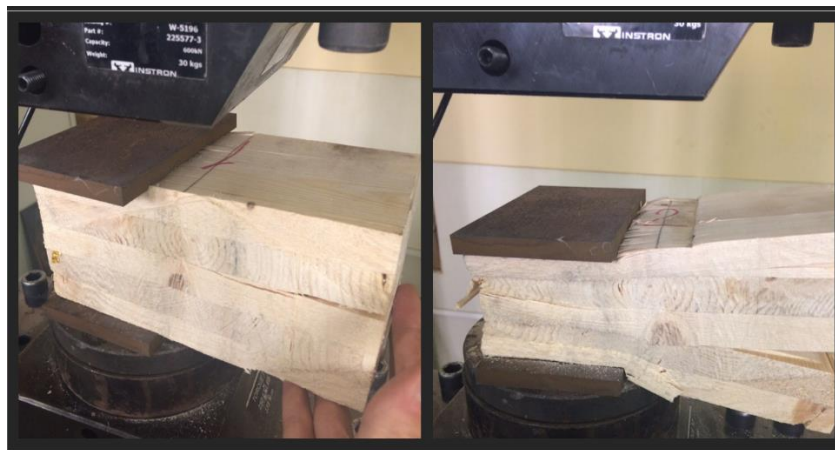
Figure 10. Modeling the support of a 5-ply floor slab on a wall panel
