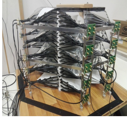
Figure 1. The S^3 detector consisting of 80 detector elements.
