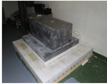
(a) Lead shielding.
