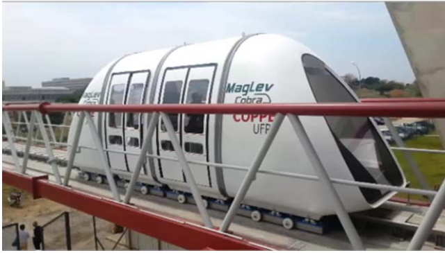
Figure 1. The Maglev Cobra on its guideway at the Federal University of Rio de Janeiro. The cryostats are visible below the vehicle. The wheels have been installed to protect the vehicle during the tests (photography by the authors).
