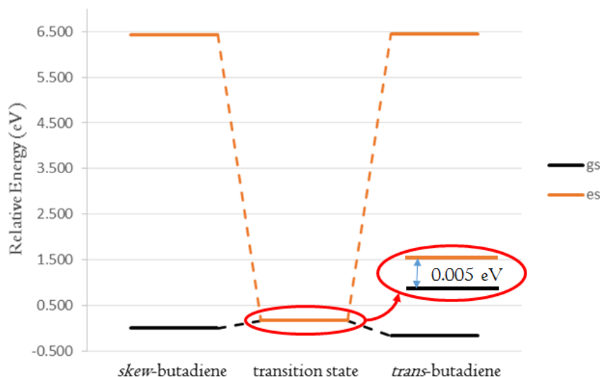
Figure 3. Energy level diagram of skew -butadiene, trans -butadiene, and the transition state connecting them in ground state (gs) and the corresponding excited state (es). The transition structure in excited state has been optimized using CASSCF method.
