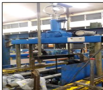
Figure 10. Pull-out testing.
