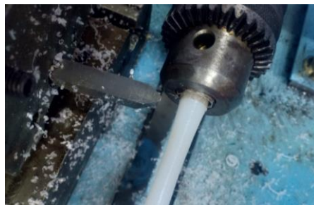
Figure 3. Special tool post for copy turning specimens profiles [16].
