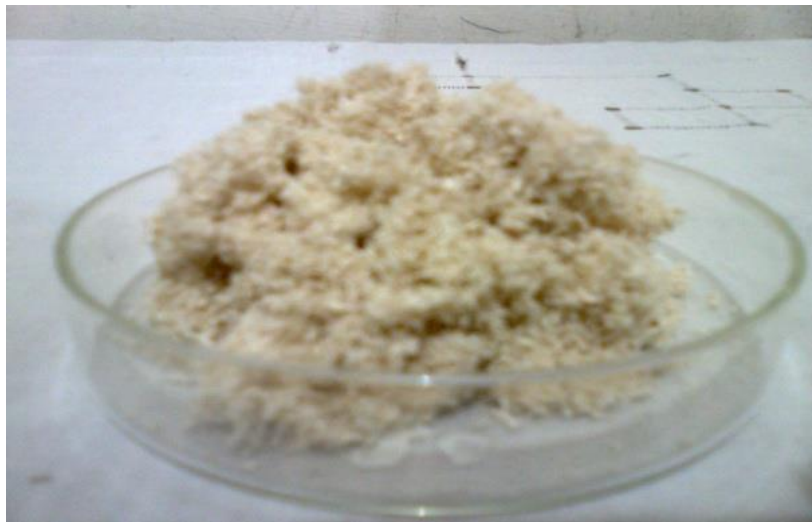
Figure 2. Empty fruit bunch fiber after bleaching.
