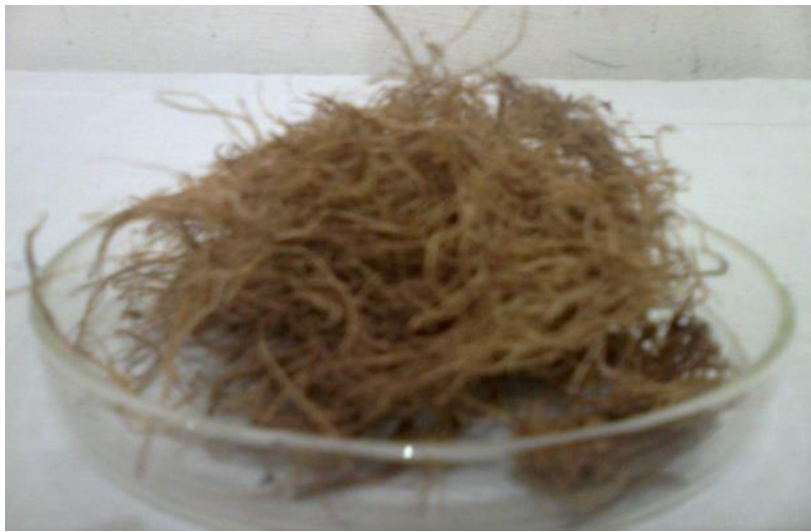
Figure 1. Original empty fruit bunch fiber.
