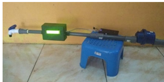
Figure 4. Water flow sensor calibration set up.
