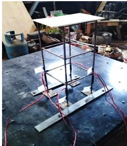
Figure 10. Specimen lay on the shaking table.
