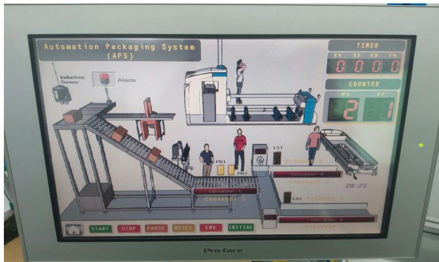
Figure 6. HMI design and implementation the automatic packaging system.
