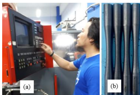
Figure 4. CNC Lathe for turning specimens profiles.
