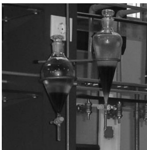
Figure 2. Layers of biodiesel and glycerol in a separating funnel.
