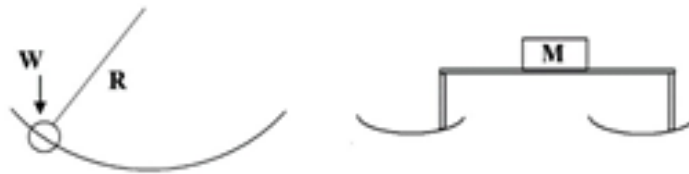
Figure 3. The concept of Base Isolator Friction Pendulum system.
