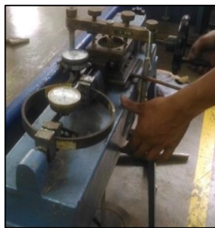
Figure 8. Direct shear test.
