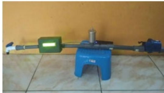
Figure 5. Air vent valve feasibility testing set up.
