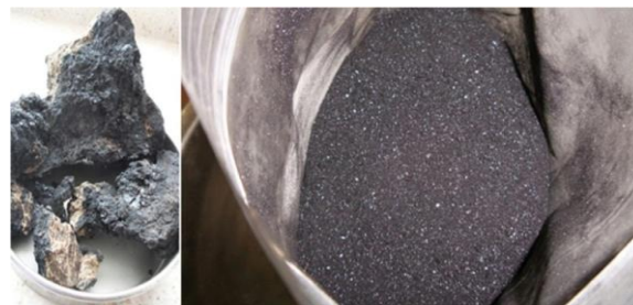
Figure 1. Gilsonite before and after milling [2].
