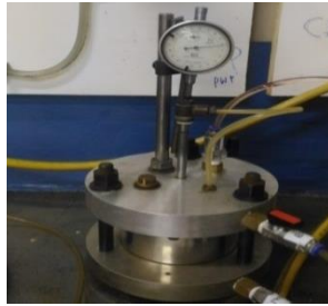
Figure 2. Set of rowe cell test.
