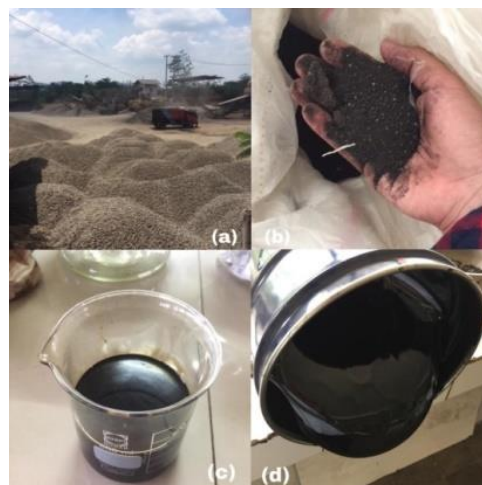
Figure 1. Materials: (a) coarse aggregate and fine aggregate; (b) 5/20 bra; (c) oily-sludge; (d) asphalt with pen 60/70.
