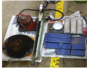
Figure 3. Set of plate loading test.
