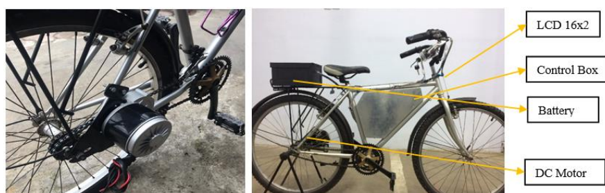
Figure 2. Design and implementation of the e-bike with 350watt DC motor mounted on rear wheel.
