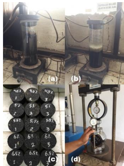
Figure 2. (a) 5/20 BRA extraction; (b) OS extraction; (c) test object; (d) marshall testing.
