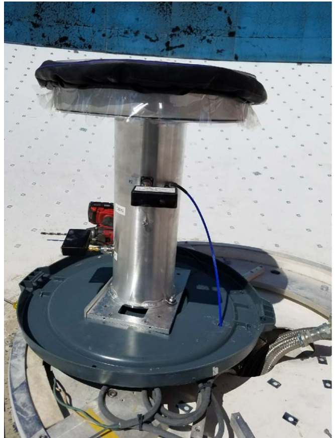
Figure 3. The choke-ring feed located at OVRO. It lies in a 6 m dish which is used as a horizon shield. The 6 m dish blocks up to 25^\circ above the horizon. (A color version of this figure is available in the online journal.)
