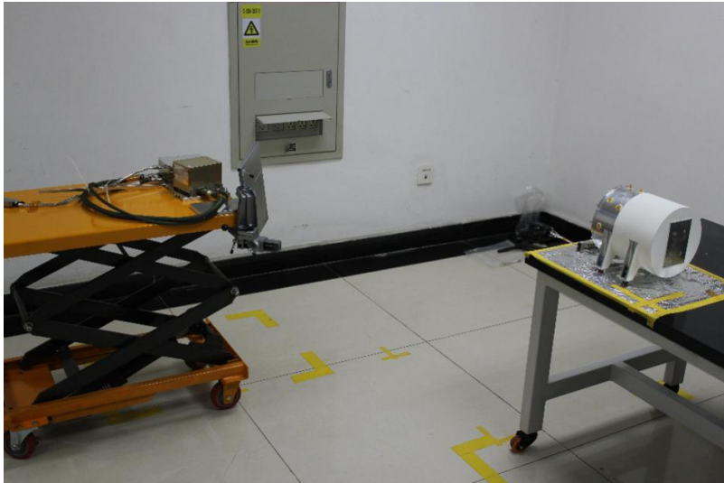
Figure 4. Test setup for the RTG in the Tianjin facility. LND is on the right of the yellow vehicle, while the RTG is set on the black laboratory table. The Al plate also on the right corner of the yellow vehicle, is mounted between the RTG and LND to mimic the shielding by the Chang'E 4 lander vehicle.
