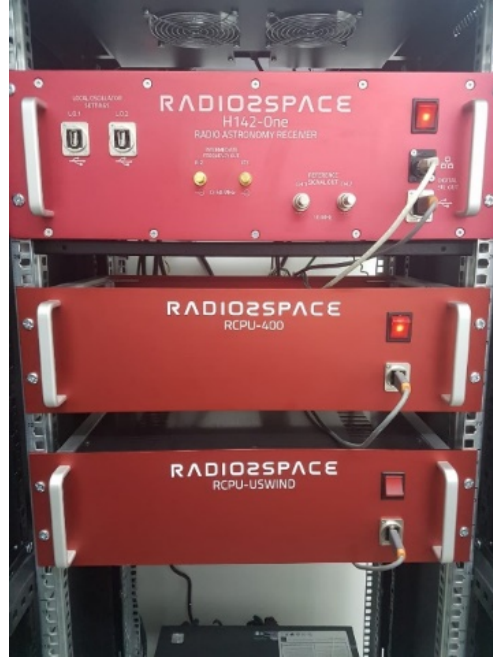
Figure 2. The H142-One radio astronomy receiver, the RCPU-400 remote control and power unit, and the RCPU-USWIND were all mounted inside a 19” computer rack.
