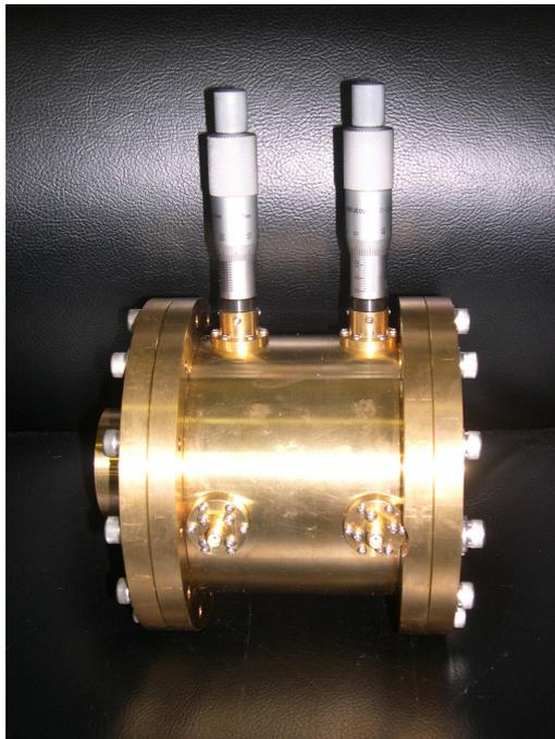
Figure 4.4: The photograph of the model cavity to check the tuning property of the gun cavity.
